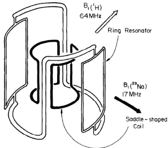
Figure: Arrangement of RF probes
