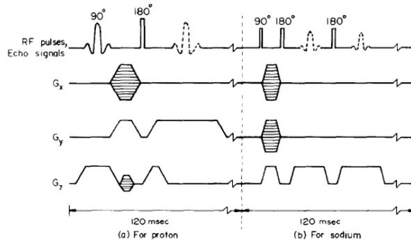
Fig. 3. Pulse sequence diagram for (a) proton and (b) sodium imaging.
