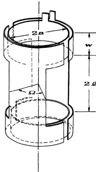
Fig. 1. The STR consisting of two foil rings, two vertical H-shaped conductors with a subtended angle of  $\Omega$  and isolation sheets (not shown).
