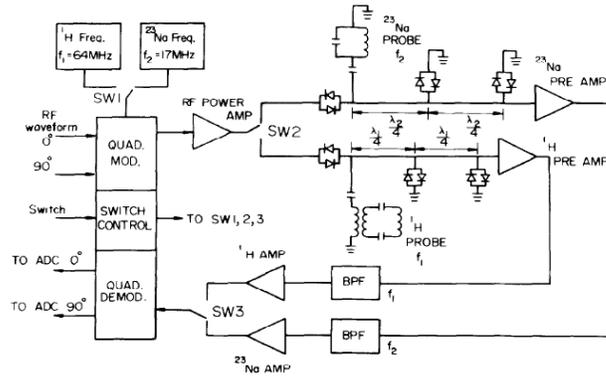
Fig. 1. Block diagram of the RF system for simultaneous multinuclear experiment.
