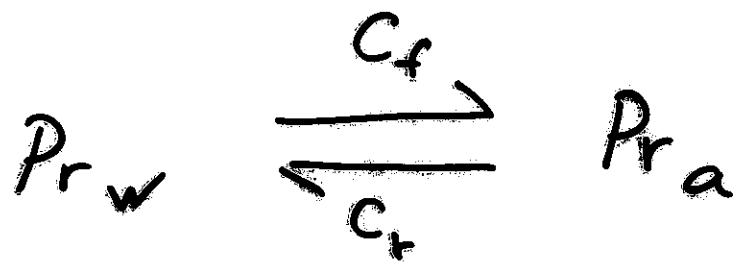
The rate of the forward reaction is equal to  $C_f [Pr_w]$  and the rate of the reverse reaction is equal to  $C_r [Pr_a]$ , for some constants  $C_f$  and  $C_r$  where the term in brackets denote concentration. Since the reverse reaction is more favorable  $C_r > C_f$ .
