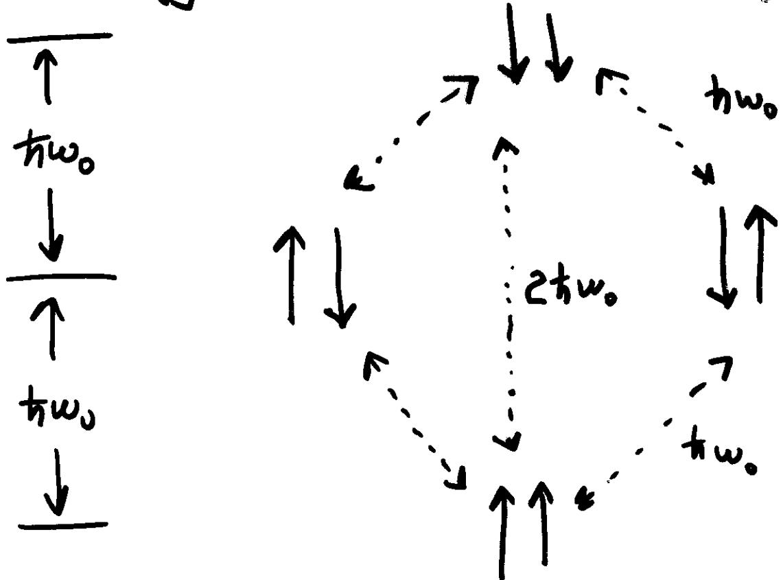
$$\frac{1}{T_1} = \frac{3}{2} \gamma^4 h^2 I(I+1) \left\{ J_1(\omega_0) + J_2(2\omega_0) \right\}$$
